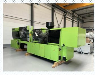
Injection Molding Machines 90Ton, 220 Ton Capacity to handle up to 3Ton Tools
